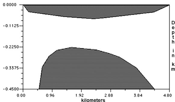
**Figure 7. Model including PlotRefa estimates for sediment thickness (top) and salt dome (bottom).**
