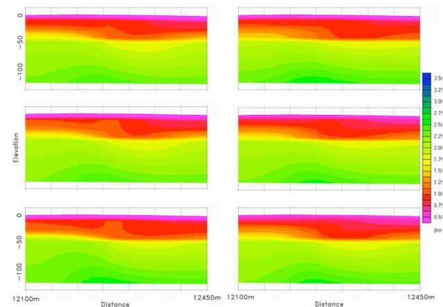
**Figure 4: Tomography results for different initial conditions. Left column: 10m, 20m, 30m depth. Right column: 40m, 60m, 100m depth.**
