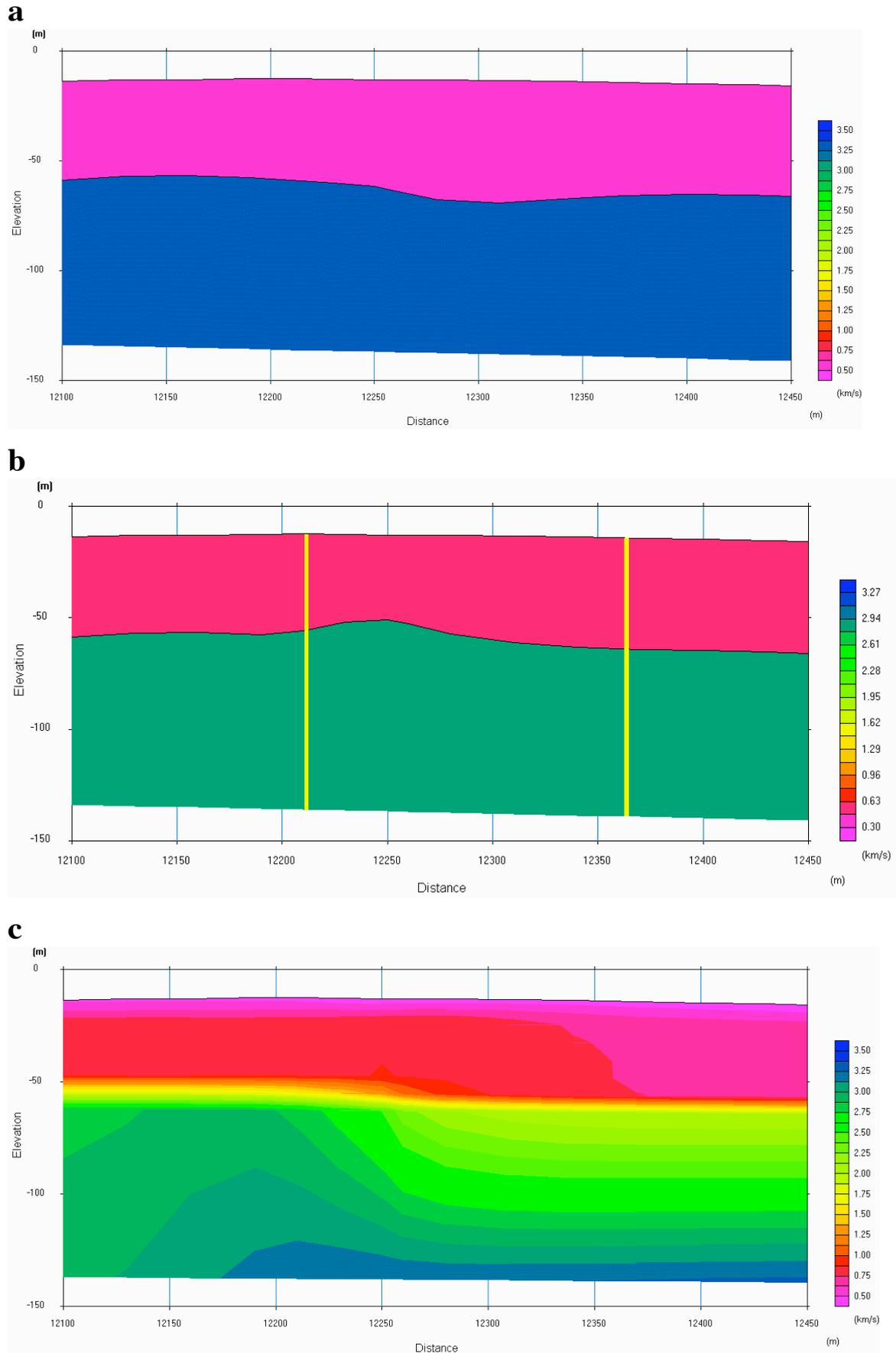
**Figure 3: Comparison of time-term method (a), reciprocal method (b), and tomographic inversion (c) for the seismic refraction line spanning survey points 12100-12450. Yellow lines indicate overlap area for the reciprocal method. Elevations are relative survey point 10000 at the southern-most end of Cyclone graben.**
